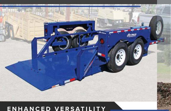
The Rental trailer is a traditional 14ft. or 16 ft. flatbed designed to benefit the rental industry. The standard features found on this trailer include: corner chain pockets, tie down bar, rear center chain slots and 2 tail end D-rings for a total of 22 different anchor points. A rubber bumper and 10" deep binder compartment are included.
