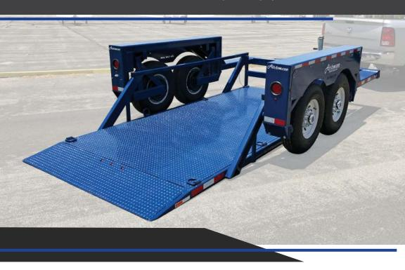
Air-tow eliminates the need for difficult tilt beds or dangerous loading ramps, making it a one man job even in adverse weather conditions. Ground-level loading is especially useful for equipment with poor traction or low ground clearance. Tandem axle models range from 7,000 to 14,000 lb. capacities. Common uses include: pavement rollers, skid steers, forklifts, etc...
