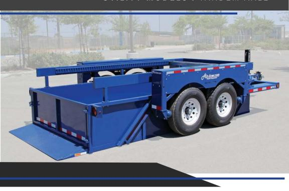
Air-tow utility models have a wide range of options to fit your exact needs. They can be customized with many accessories such as E-tracks, tailgates and extended rails. Tandem axle utility models range from 7,000 to 14,000 lb. capacities. Common uses include: safes, vending machines, skid steers, etc.
