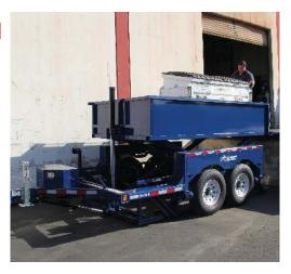
■ 5ft Dock Height Loading ■ 8 Heavy Duty D-Rings ■ 74" Deck Width ■ Folding Ramp
