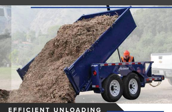
This hybrid trailer lowers flat to the ground for safer, easier and faster loading and unloading as well as being a full-blown dump trailer. With a load capacity of 10,000 lbs and a dump capacity of 8,000 lbs, the "3D" trailer is ideal for moving your skid steer to the job site then loading and hauling debris. With a dual fold-down/spreader tailgate, you have the option of
