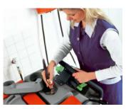
Automatic dosing and and filling system: Saves time when filling the tank, and the reduced consumption of cleaning detergents saves on operating costs.
