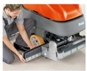
No pre-sweeping required, thanks to the integrated and easy-to-empty coarse dirt tray at the cylindrical brush unit.
