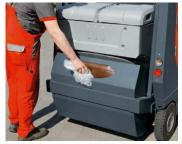
Practical coarse dirt flap to throw-in larger piecesof debris, plastic films or straps. No dust can escape when opening the coarse dirt flap.
