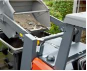
**Hydraulic High-Dump Option:** The dirt hopper allows high dumping at heights of up to 60".
