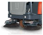
Robust chassis and collision protection: The chassis provides a solid base and collision-protected brooms ensure highest possible machine reliability.
