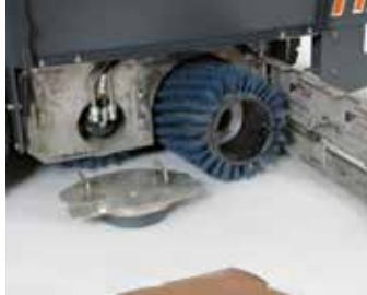
Easy changing of the brushes: Thanks to the quick-change system, changing the cylindrical brushes is particularly easy, no tools needed.
