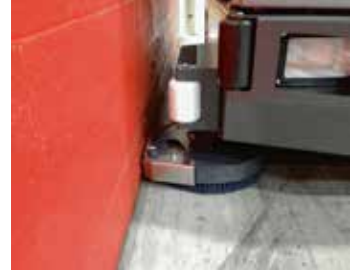
Working close to edges: The optional side scrub unit allows cleaning right up to walls.
