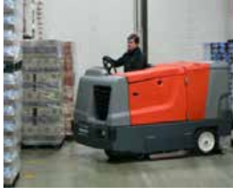
Working in confined areas: PowerBoss Nautilus has a small turning circle. This machine can make a complete U-turn in aisles as narrow as 108 inches, allowing the operator to keep an eye on the surrounding traffic at all times.
