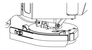
Fig. 1: Replacing the Side Scrub Brush
