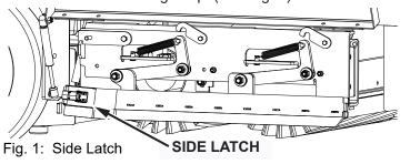
5. Replace the side squeegee blade by placing the blade onto the pins of the side squeegee frame.
