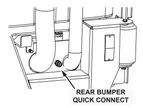
Fig. 1: Spray Wand Quick Disconnect
