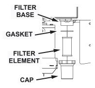
Fig. 2: Water Solution Filter with Exploded view
