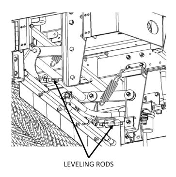
Fig. 4: Leveling Rod location
