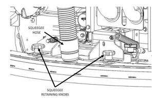
Fig. 1: Turning/Replacing the Rear Squeegee Blades
