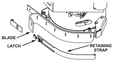
Fig. 3: Retaining Strap & Blade
