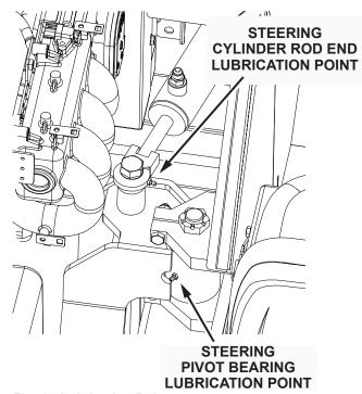
Fig. 1: Lubrication Points
