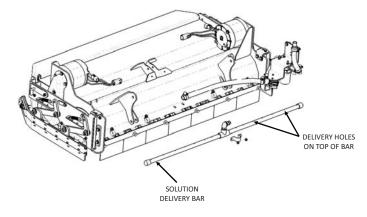
Fig. 1: Solution Delivery Bar shown with holes
