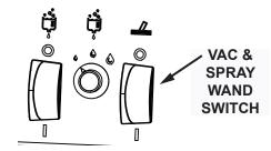
Fig. 2: Vacuum and Spray Wand Switch
