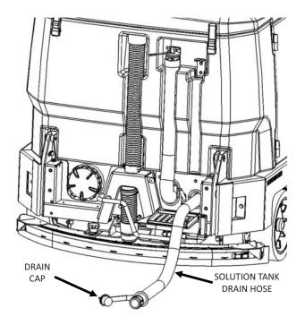
Fig. 1: Draining the Solution Tank
