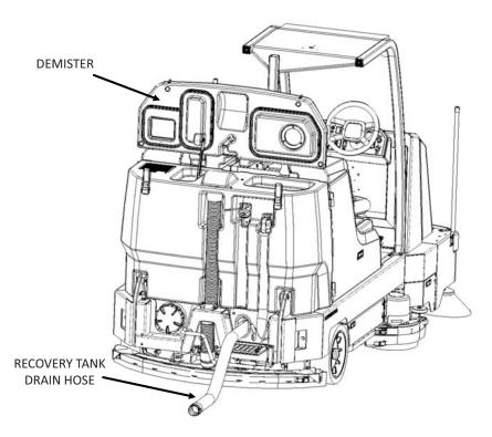
Fig. 1: Draining the Recovery Tank
