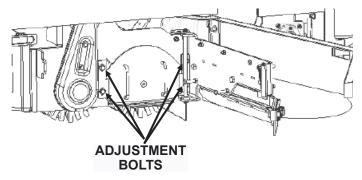
Fig. 2: Adjustment Bolts, location
