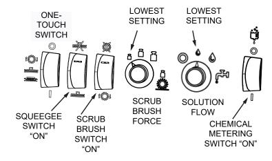
Fig. 1: Control Settings, before "One-Touch" selection
