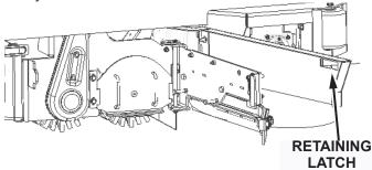
Fig. 1: Retaining Latch location
