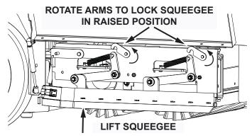
Fig. 1: Shows squeege assembly retaining arms
