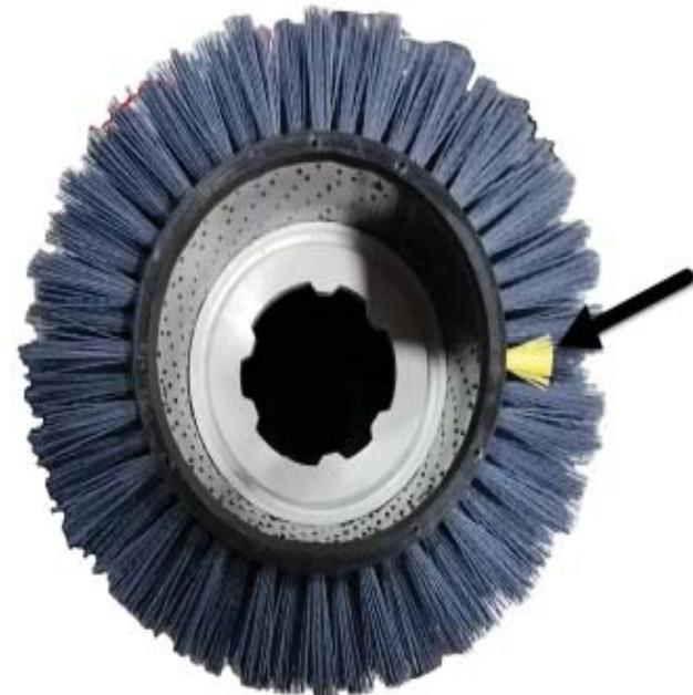
6. Grasp the main broom by the plastic drive hub, pull the main broom straight out and clear of the broom chamber.
