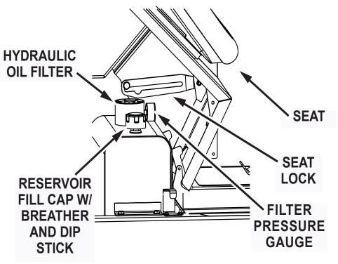
Fig. 2: Hydraulic Fluid Reservoir location
