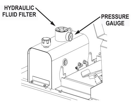
Fig. 2: Hydraulic Filter & Pressure Gauge
