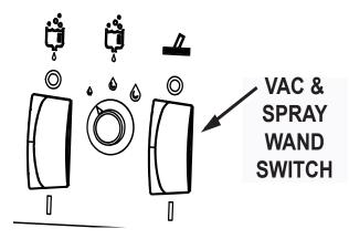
Fig. 2: Vacuum and Spray Wand Switch
