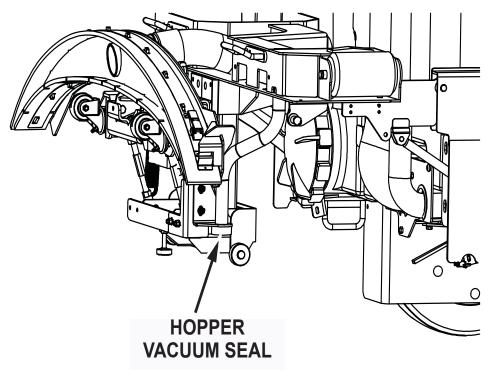
Fig. 3: Hopper Vacuum Seal location
