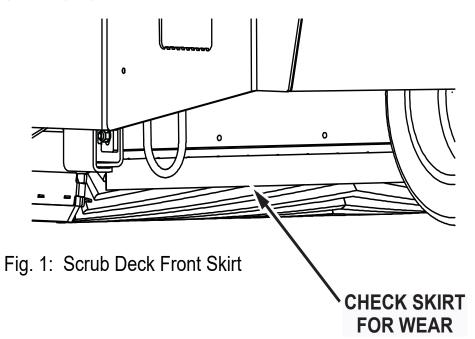
Check this skirt for wear or damage every 100 hours of operation.
