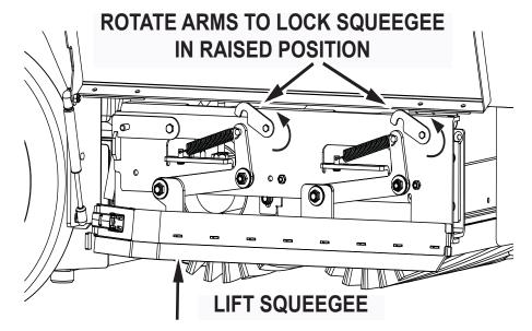
Fig. 1: Shows squeege assembly retaining arms
