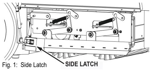
5. Replace the side squeegee blade by placing the blade onto the pins of the side squeegee frame.
