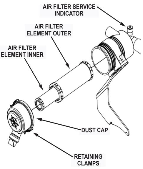
Fig. 1: Air Intake System
