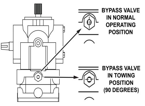
Fig. 2: Bypass Valve locations
