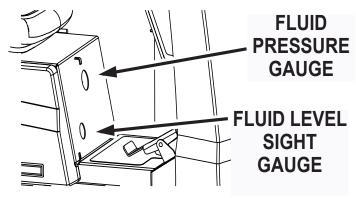
Fig. 3: Hydraulic Fluid Gauges
