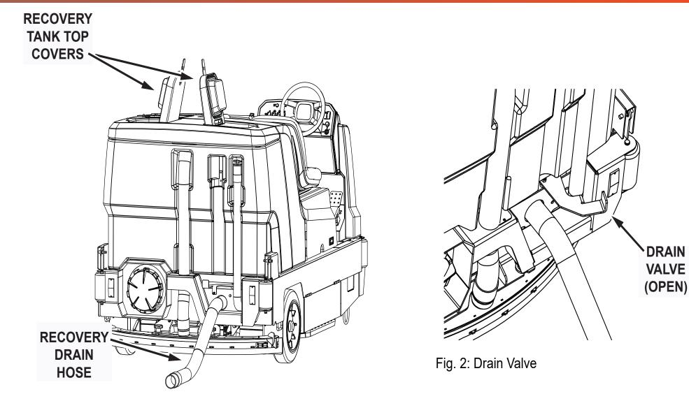
Fig. 1: Draining the Recovery Tank
