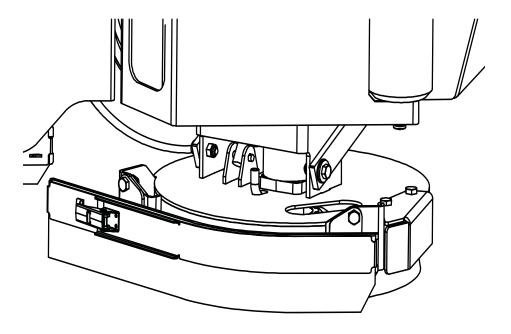
Fig. 1: Replacing the Side Scrub Brush
