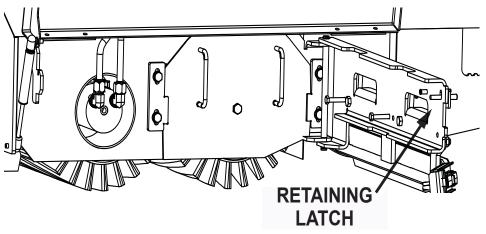
Fig. 1: Retaining Latch location
