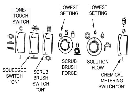
Fig. 2: Control Settings, before "One-Touch" selection
