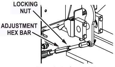
Fig. 2: Brake System Adjustment
