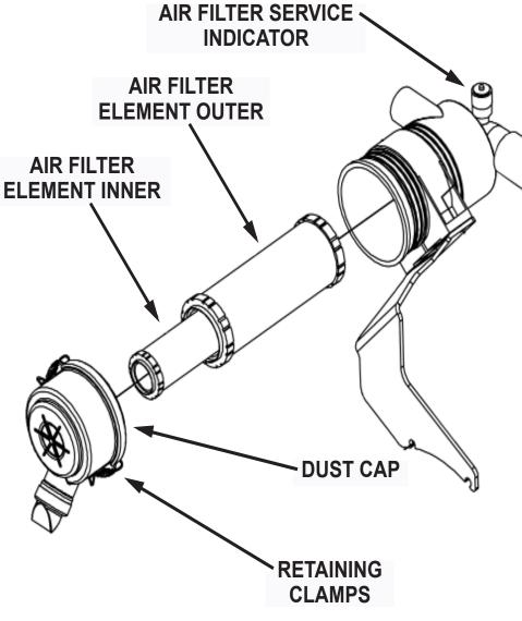
Fig. 1: Air Intake System
