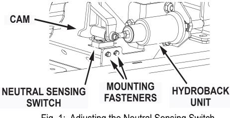
Fig. 1: Adjusting the Neutral Sensing Switch
