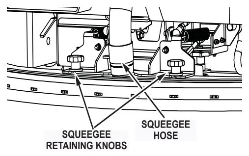
Fig. 1: Turning/Replacing the Rear Squeegee Blades
