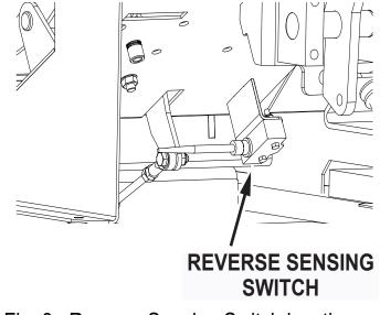
Fig. 3: Reverse Sensing Switch location
