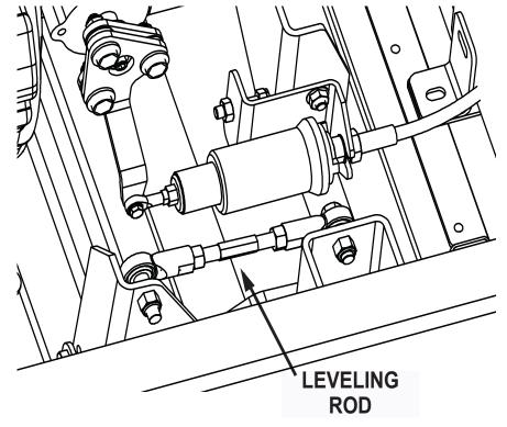
Fig. 4: Leveling Rod location
