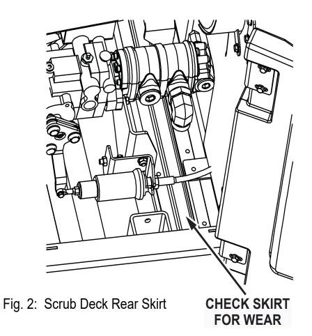
Check this skirt for wear or damage every 100 hours of operation.
