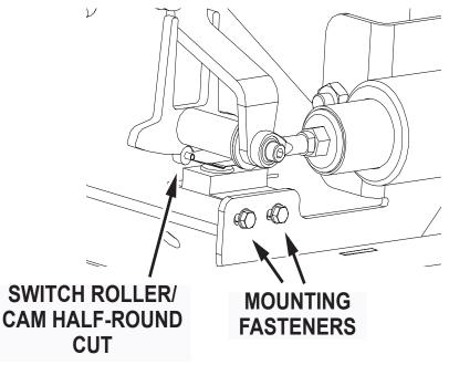
Fig. 2: Roller and Cam Position
