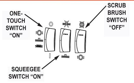
Fig. 1: Control Settings for Water Pick-up Mode
