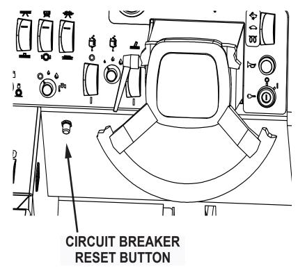
Fig. 1: Circuit Breaker location
