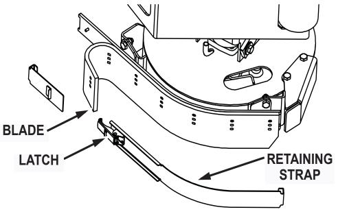
Fig. 3: Retaining Strap & Blade
