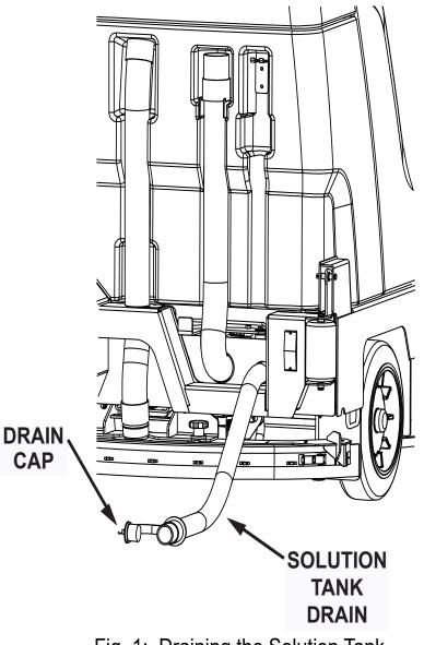
Fig. 1: Draining the Solution Tank
