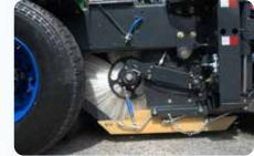
LONG LASTING DIRT SHOES • Polyurethane Dirt Shoes are designed so that operator has sweep over potholes and rail road tracks and will not damage while sweeping. Long Life of 1000 hours is guaran-teed. 47" Gutterbrooms assist in cleaning curbs and heavy Road Millinas.
