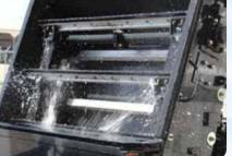
HEAVY SWEEP PACKAGE • Elevator Type: Standard 11 Flight squeegee with replaceable corded rubber tips; Con-tinuous molded rubber belts combine with standard Heavy Sweep Package make Electric Global M4 the logical choice for sweeping heavy debris such
