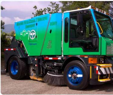
With travel speed of 55-MPH and a battery operational range of up to 11 hours, towns, villages and large cities will be able to clean the streets while protecting our environment and building a cleaner future with ZERO EMISSIONS. At the end of the shift just plug in the sweeper, recharge the batteries and sweep again.
