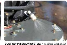
includes 230 Gallon Water Tank Capacity combined with Two(2) Diaphragm Water pumps and Two(2) Modes (LOW/HIGH) provide versatility and superb dust control
