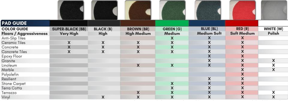
\*Recommended rpm range for scrubbing pads is 175 - 350 rmp, and should be used wet.
