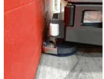
Working close to edges: The optional side scrub unit allows cleaning right up to walls.
