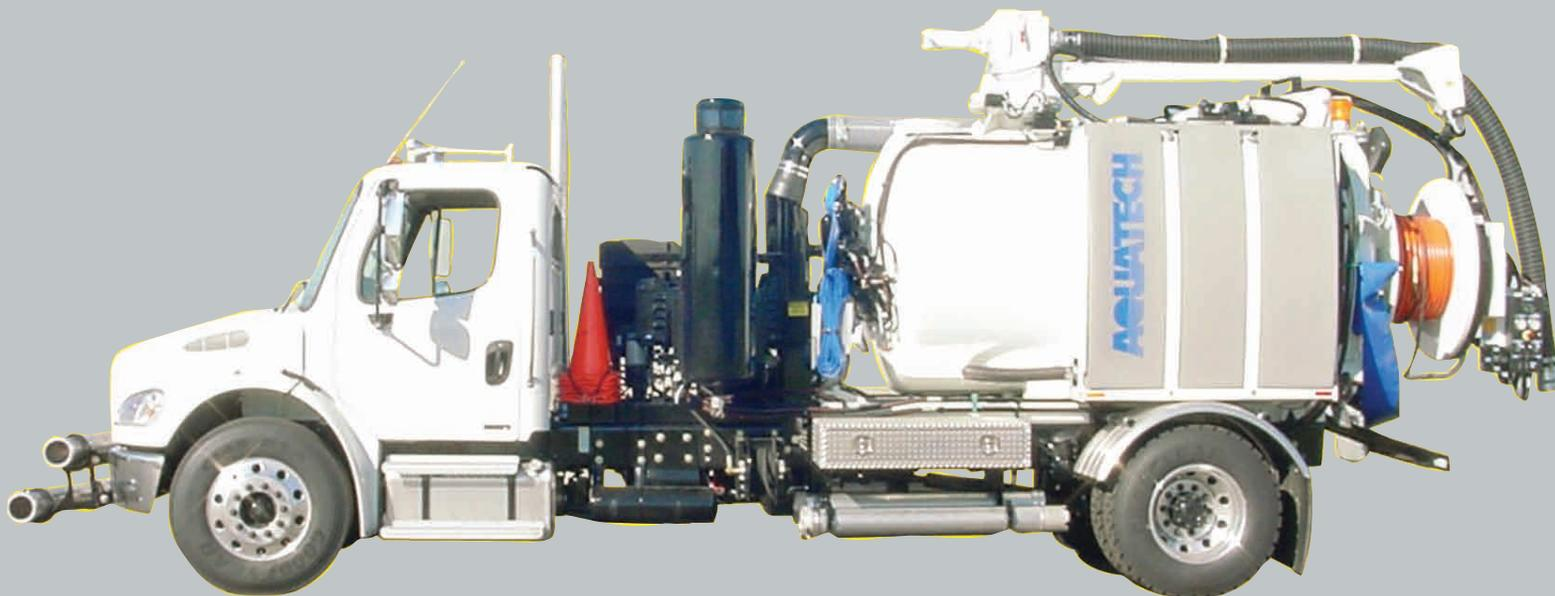
The B6 Combination Cleaners are designed to give unsurpassed performance in catch basins, storm sewers, lift stations and treatment plants in municipal and industrial applications.
