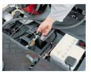
Adjusting the brooms: Central adjustment of the brooms; no tools needed.
