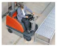
Maneuverability: Small turning circle even in particularly confined areas thanks to the 90-degree steering angle.
