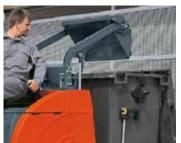
**Comfortable high dump:** At the push of a button, the dirt hopper can be emptied directly into any customary waste container (option).
