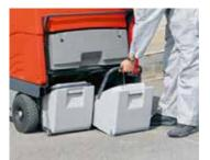
Take-it-easy: The two dirt hoppers can be removed separately and emptied with ease. The hopper lifting system is particularly easy to operate and allows checking the filling level or throwing coarse pieces of debris into the hoppers at any time.
