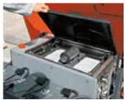
Filter: Easy-to-access electric R<sup>2</sup>S filter shaker system.
