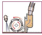
Three spray jets force solution into carpet; independently powered brush deep cleans; and powerful vacuum picks up all the dirty solution to leave carpet clean and virtually dry.
