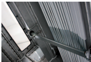
Dulevo Patented Mechanical-suction-filter system
