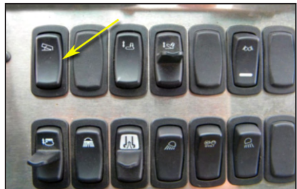
HOPPER DUMP SWITCH
