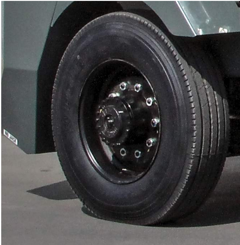
Fig. 2.7 – Each rear wheel torque hub must be disengaged before sweeper can be towed. Remove towing plate and remount with dimple facing inward disengaging torque hub.
