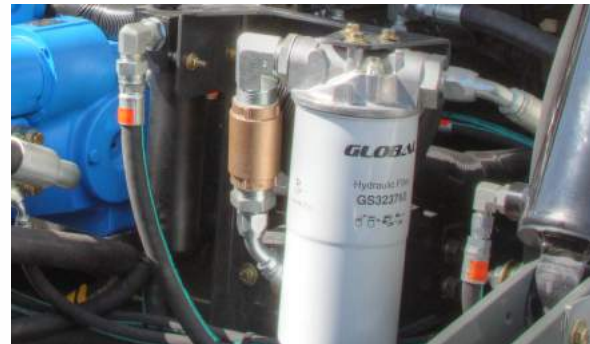
Fig. 4.4 – Hydraulic suction and high pressure line filters are equipped with gauges which monitor flow performance. Suction filter and gauge is located on right side of engine compartment. High pressure line filter and gauge is located on left side of engine compartment. Check filter gauges with engine/hydraulic oil warm.
