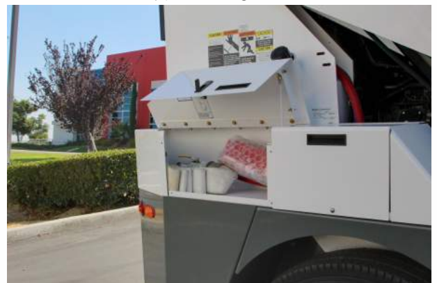
Fig. 2.4 – Fire hydrant filler hose and related tools are located in right rear fender tool box.
