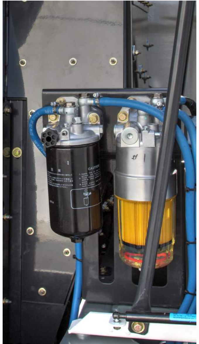
Fig. 4.6 – Primary fuel filter is mounted on inside wall of right hydraulic tank. When replacing, fill new filter with fuel before installing. Secondary fuel filter system is located on right side of engine block.
