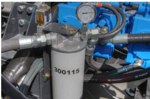
Fig. 4.4 – Hydraulic suction and high pressure line filters are equipped with gauges which monitor flow performance. Suction filter and gauge is located on right side of engine compartment. High pressure line filter and gauge is located on left side of engine compartment. Check filter gauges with engine/hydraulic oil warm.
