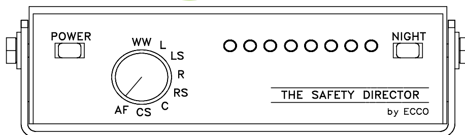
FRONT VIEW OF CONTROL BOX
