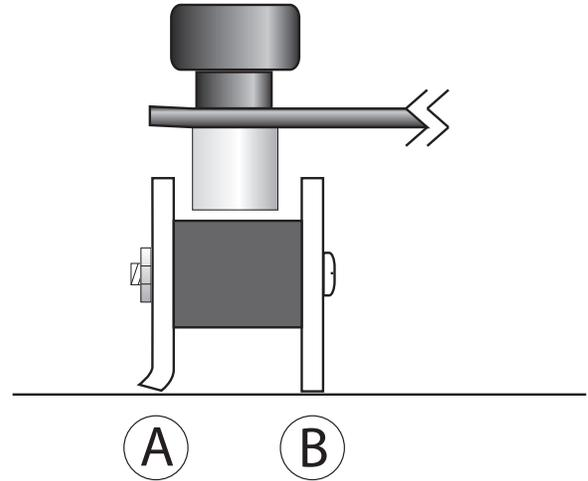
Properly Adjusted Squeegee: Front blade just contacts the floor rear blade is slightly flared outward
