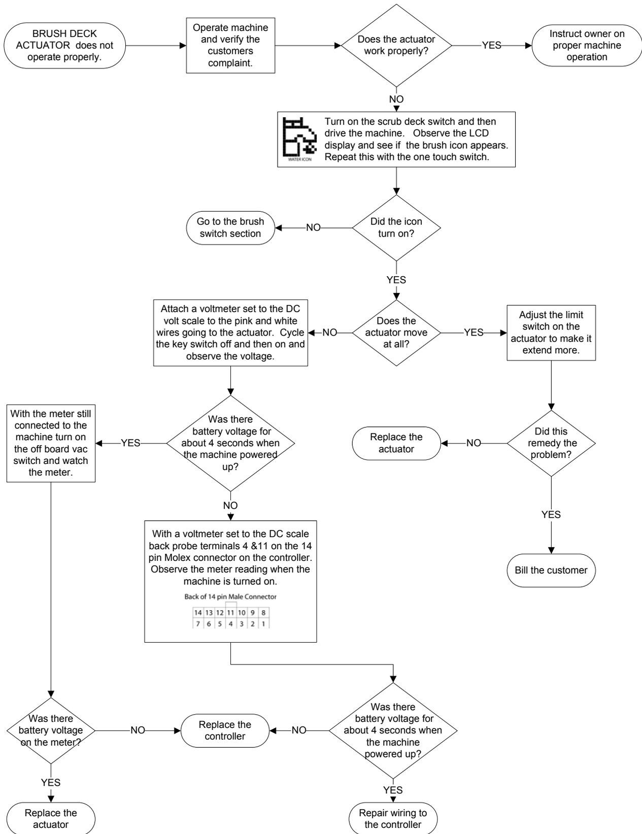
**XR SERIES BRUSH PRESSURE SWITCH DIAGNOSTIC FLOW CHART**
