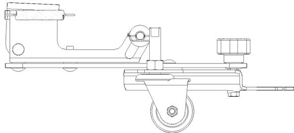
Turning the knob clockwise lowers the front blade of the squeegee thereby closing off the air holes against the floor. This increases suction on the floor. If you adjust it too far forward you can cause chattering problems, excessive front squeegee blade wear or grind the tips off both the front and rear squeegee blades.
