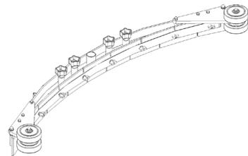
A suspension that mounts the squeegee to the machine, and allows the squeegee to move up and down with variations in the floor, and pivot in turns.
