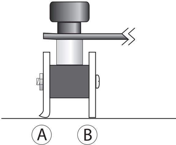
Worn Blade: Squeegee wiping edge has worn so the square edge is gone. The squeegee now runs over the water instead of scraping it off the floor.
