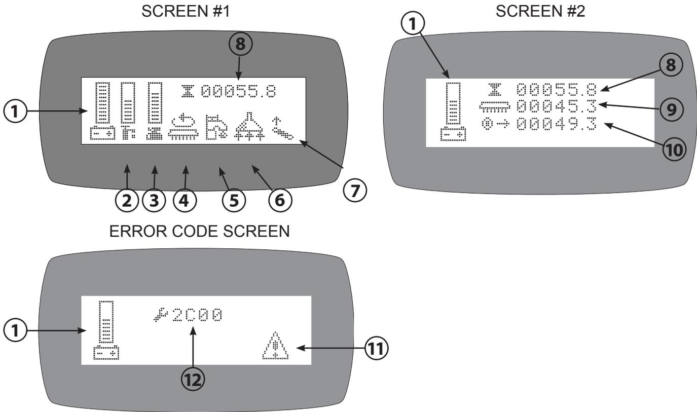
TO CHANGE CYCLE THROUGH SCREENS 1 and 2 USE THE GREEN PAGE BUTTON NEXT TO THE LCD DISPLAY. THE ERROR CODE SCREEN ONLY APPEARS WHEN THERE IS A PROBLEM WITH THE MACHINE.
