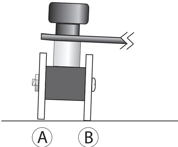
Too Much forward pitch on this squeegee. The Rear blade is barely making contact with the floor. The rear wheel are not touching the floor.
