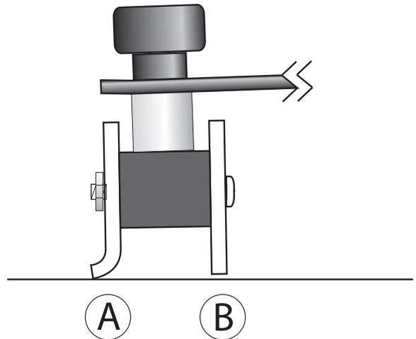
Too Much backward pitch on this squeegee. The rear blade is laying over and the front blade is not touching the floor.
