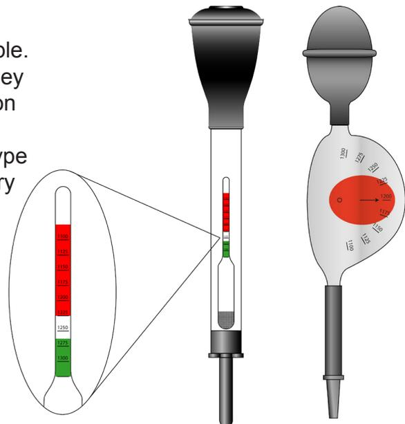
The state-of-charge of a lead acid battery can be determined by the specific gravity of the electrolyte (its weight compared to water). The specific gravity can be measured directly with a hydrometer or determined by the stabilizing voltage.
