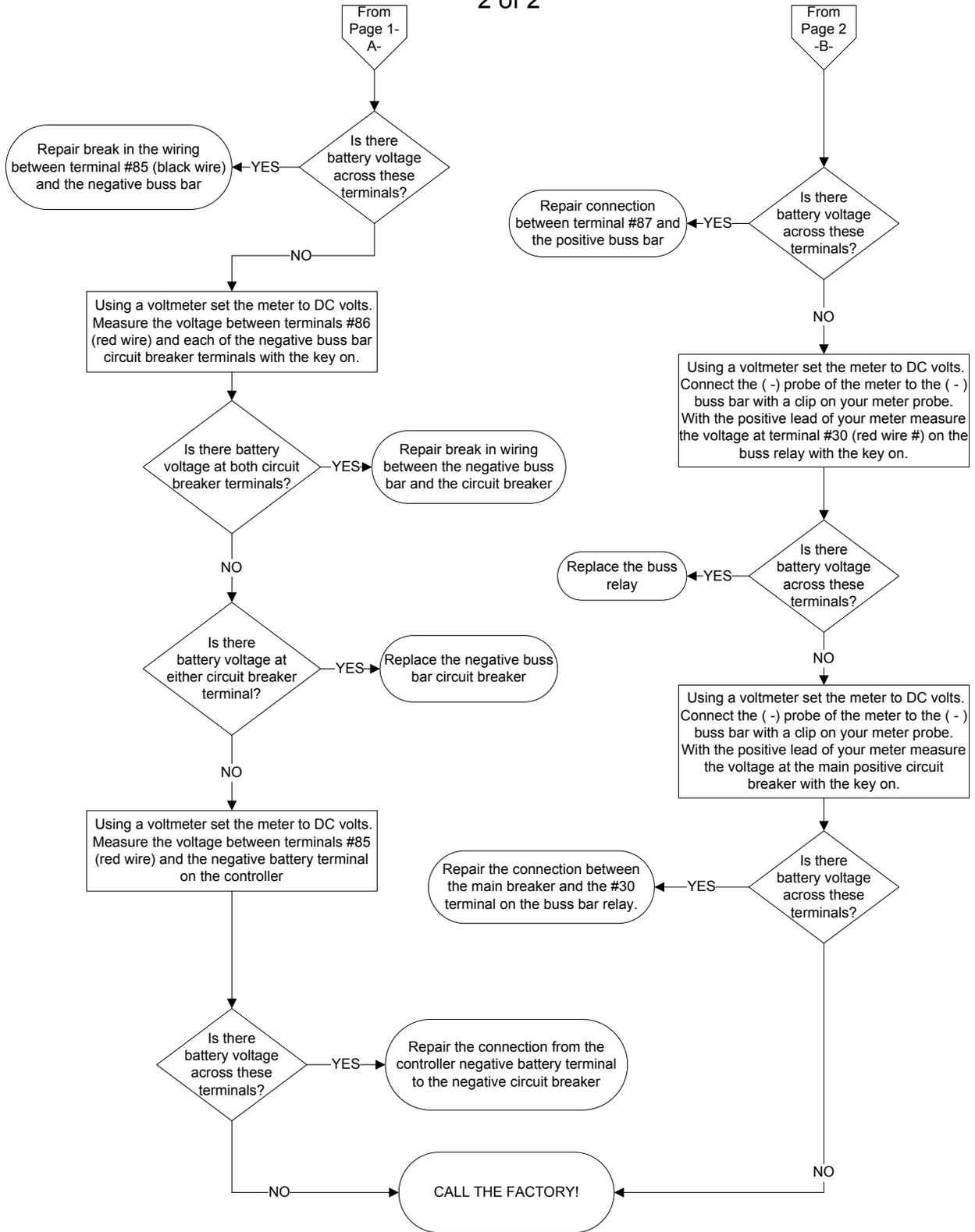
**XR SERIES SOLUTION SOLENOID VALVE DIAGNOSTIC FLOW CHART**
