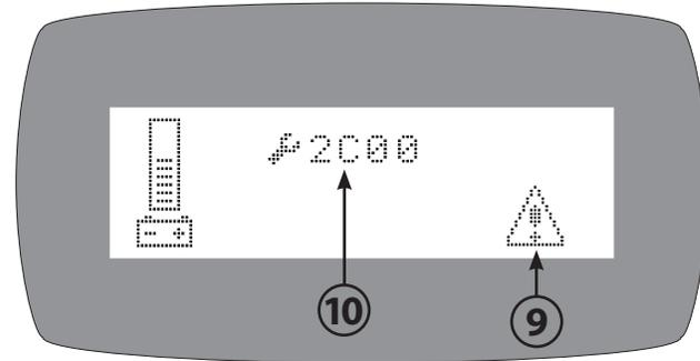
TO CHANGE CYCLE THROUGH SCREENS 1-3 USE THE GREEN PAGE BUTTON NEXT TO THE LCD DISPLAY. THE ERROR CODE SCREEN ONLY APPEARS WHEN THERE IS A PROBLEM WITH THE MACHINE.
