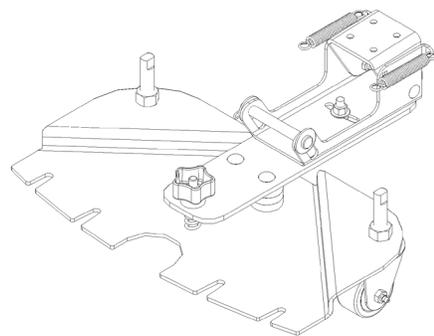
A lift system that allows the operator to raise the squeegee off the floor. The machine has a fully automatic electric lift system.
