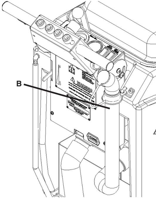
3. Flush Recovery Tank with water hose.
