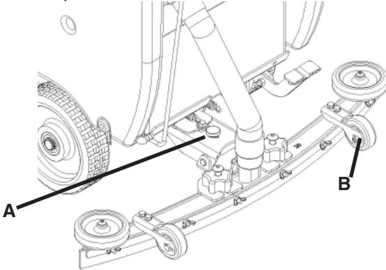
2. Adjustable Wheel **(B)** (**SEE ABOVE**) has 3 holes. The closer to the machine the wheel is, the further from the ground the wheel becomes. The farther from the machine the wheel is, the closer to the ground the wheel becomes.
