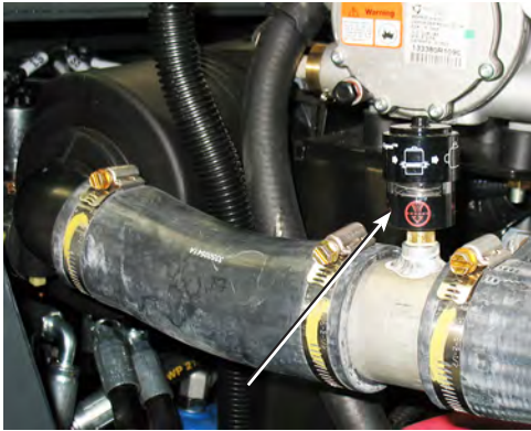
Air Mechanical Vacuum Filter Service Indicator Location
