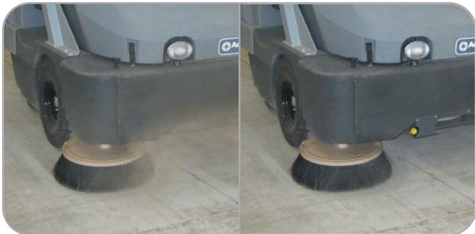
DustGuard™ suppresses airborne fugitive dust allowing continuous use, and increasing productivity by up to 71%.
