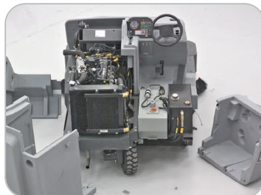
MaxAccess allows faster repairs and less downtime so the sweeper spends less time in the shop and more time sweeping.
