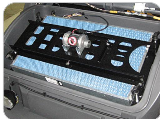
Ultra-Web® dust filter is >98% efficient on 0.3 - 1 micron dust. This meets MERV 13 on the ASHRAE 20 point scale.
