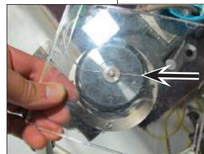
The wire rotates with the magnetic field as the steering wheel rotation sensor shaft is turned
