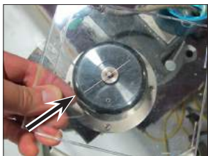
The wire rotates with the magnetic field as the steering wheel rotation sensor shaft is turned
