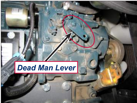
Dead man lever in normal run position
