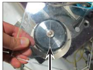
The wire rotates with the magnetic field as the steering wheel rotation sensor shaft is turned
