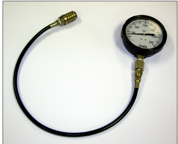
Hydraulic test gauge w/connector 3000 psi range, p/n 56504516
