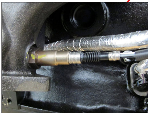
Upstream (Pre-CAT) O 2 Sensor
