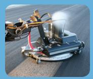
Chemical and vacuum free cleaning removes and recovers rubber and paint build-up in a single pass.
