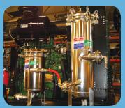
Organic materials and particles filtered from water to 0.35 microns.
