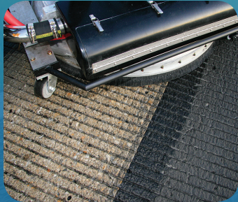
Cleans into the grooves of a runway for increased friction and drainage.
