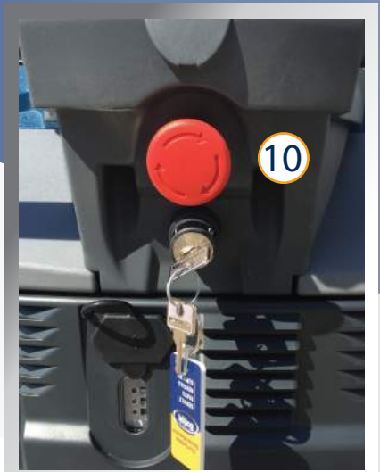
The 500 RSX and SS come with an emergency shut-off button for immediate cease of operation.
