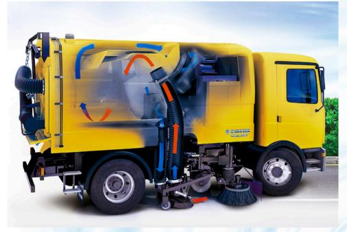
"Patented Sweeping System" Our Air Recirculation Technology (VAST) allows for sweeping below freezing conditions while expelling 50% less fine dust emission compared to a pure vacuum concept.
