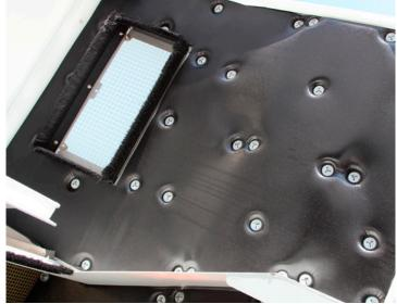
**SILENT PLUS PACKAGE QUIET SWEEPING OPERATION** The **"Silent Plus"** option utilizes sound supressive material in the engine compartment effectively reducing noise pollution during sweeping to 87 dB(A).
