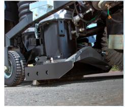
**THE "V-NOZZLE" WILL SWEEP IT ALL** The V-shaped Suction Nozzle with its large aperture, made of 4mm steel, conveys the swept material directly into the suction tube. This design enables the **Global V6AIR** to lift the Heaviest of debris in any application.
