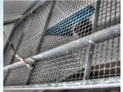
The **Global V6AIR** includes **Galvanized Hopper Screens** that can be easily lowered for cleaning without raising the hopper. The Screening system is designed so that Hopper Screens do not plug up when sweeping light debris such as leaves.
