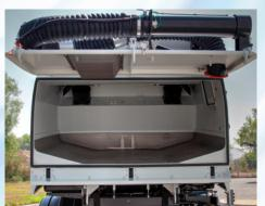
QUALITY, BUILT TO LAST STAINLESS STEEL CONSTRUC-TION Hopper Design includes only the best such as 304 Grade Stainless Steel (100%) integrated into the 8.5 Cu.Yd. Hopper.
