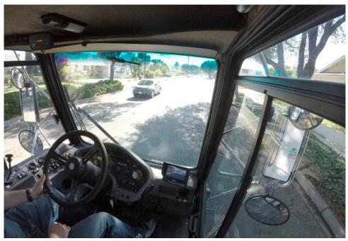
The inherent design of the **Global M4HSD** makes it the logical choice among 4-wheel mechanical sweepers. With the center mounted/cab forward layout the operator has unsurpassed visibility of the road surface as well as pedestrians and surrounding traffic. The large hopper capacity equals more lane miles swept between dump cycles and the 18.5-foot turning radius makes the **Global M4HSD** highly efficient and comfortable.
