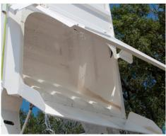
LARGEST USEABLE CAPACITY IN IT'S CLASS Global M4HSD includes a 5.2 culyd hopper capacity compared to 4.5 culyd on competitive machines resulting in more curb miles swept between dump cycles. With near Full Useable Capacity, 12,000-LB Lift Capacity, and the Optional Elevator Wash Out System, Global M4HSD is Affordable, Reliaible and innovative.
