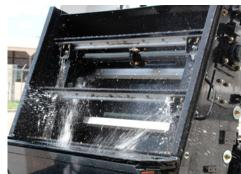
HEAVY SWEEP PACKAGE Elevator Type: Standard 11 Flight squeegee with replaceable corded rubber tips; Continuous molded rubber belts combine with standard Heavy Sweep Package make Global M4HSD the logical choice for sweeping heavy debris such as road millings, sand and gravel up to 3-tons per-minute. That is one ton every 20 seconds! Standard leaf gate system assists in picking up large debris, bottles, large branches and leaves.
