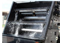
HEAVY SWEEP PACKAGE Elevator Type: Standard 11 Flight squeegee with replaceable corded rubber tips; Continuous molded rubber belts combine with standard Heavy Sweep Package make Global M4 the logical choice for sweeping heavy debris such as road millings, sand and gravel up to 3-tons per-minute. That Is one ton of sand every 20 seconds! Standard leaf gate system assists in picking up large debris, bottles, large branches and leaves.
