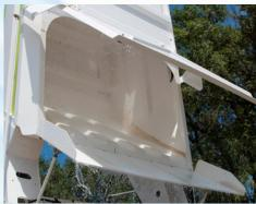
LARGEST HOPPER IN IT'S CLASS The Global M3 includes a 5.6 culyd hopper capacity compared to 3.5 culyd for competitive machines resulting in more curb miles swept between dump cycles. With near Full Useable Capacity, 12,000 Lift Capacity, and the Optional Hopper Wash Out System, Global M3 is Affordable, Reliable and innovative
