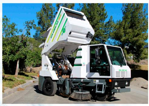
**SIMPLY MAINTAINABLE** The Global M3 is designed to make routine maintenance easy, so your sweeper spends more time on the street and less time in the garage. Two swing-out center body panels provide unrestricted access for elevator adjustment, maintenance and daily cleaning.
