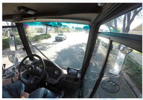
The inherent design of the **Global M3** makes it the logical choice among 3-wheel mechanical sweepers. With the center mounted/cab forward layout, the operator has un-surpassed visibility of the road surface as well as pedestrians and automotive traffic. The industry leading hopper size provides more lane miles swept between dump cycles and 12.5-foot turning radius makes the **Global M3** highly-efficient and comfortable to operate.
