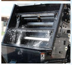
**HEAVY SWEEP PACKAGE** Elevator Type: 11 Flight squeegee with replaceable corded rubber tips; Continuous molded rubber belts and a Direct drive Hydraulic Motor: Optional ELEVATOR WASH-OUT System sigificatly reduces end of day cleaning for the operator.
