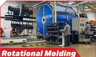
Complex shapes that allow for our "tank-in-tank" design are best achieved with in-house equipment. We own multiple dual station rotational molding machines that allow us to produce finished parts from raw plastic. Producing consistently higher
