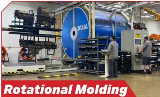
Complex shapes that allow for our "tank-in-tank" design are best achieved with in-house equipment. We own multiple dual station rotational molding machines that allow us to produce finished parts from raw plastic. Producing consistently higher quality parts and respond quickly to sales spikes.
