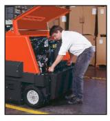
Easy access to engine makes maintenance and service repair easy.
