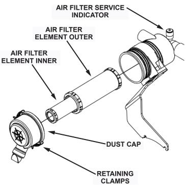
Fig. 1: Air Intake System
