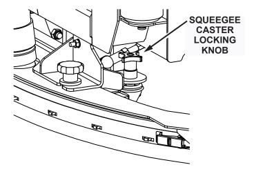
Fig. 1: Adjusting the Rear Squeegee Blade Flair
