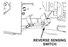
Fig. 3: Reverse Sensing Switch location
