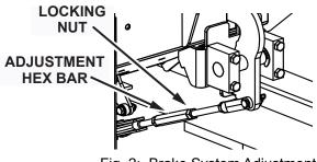
Fig. 2: Brake System Adjustment
