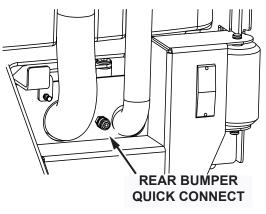
Fig. 1: Spray Wand Quick Disconnect
