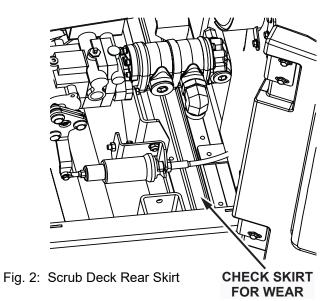
Check this skirt for wear or damage every 100 hours of operation.
