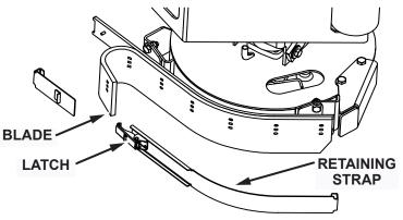
Fig. 3: Retaining Strap & Blade
