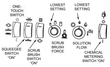
Fig. 2: Control Settings, before "One-Touch" selection
