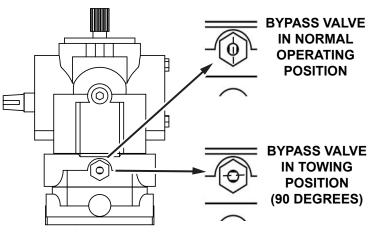
Fig. 2: Bypass Valve locations
