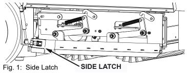
5. Replace the side squeegee blade by placing the blade onto the pins of the side squeegee frame.
