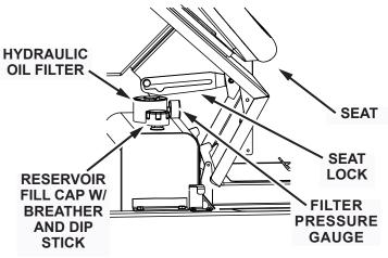
Fig. 2: Hydraulic Fluid Reservoir location
