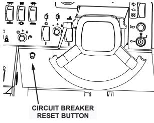
Fig. 1: Circuit Breaker location
