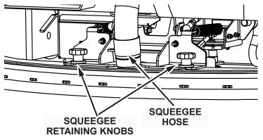
Fig. 1: Turning/Replacing the Rear Squeegee Blades
