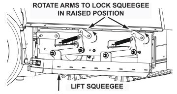
Fig. 1: Shows squeege assembly retaining arms
