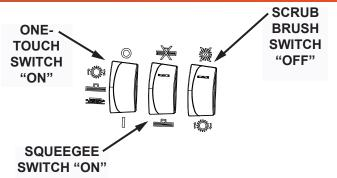
Fig. 1: Control Settings for Water Pick-up Mode
