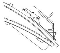
Fig. 3: Closing the Latches
