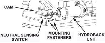
Fig. 1: Adjusting the Neutral Sensing Switch
