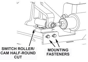
Fig. 2: Roller and Cam Position
