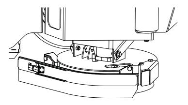
Fig. 1: Replacing the Side Scrub Brush
