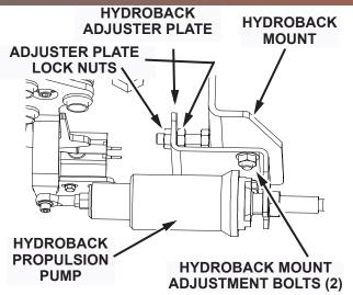
Fig. 1: Hydroback Propulsion Pump
