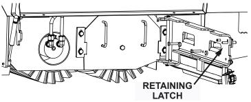
Fig. 1: Retaining Latch location
