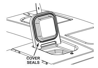
Fig. 3: Hopper Vacuum Seal location
