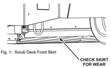
Check this skirt for wear or damage every 100 hours of operation.
