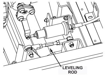
Fig. 4: Leveling Rod location
