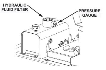
Fig. 2: Hydraulic Filter & Pressure Gauge
