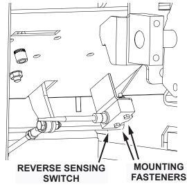
Fig. 1: Reverse Sensing Switch Fasteners
