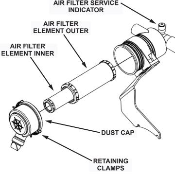
Fig. 1: Air Intake System
