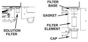
Fig. 2: Water Solution Filter with Exploded view Nautilus Rider Scrubber/Sweeper #988749UM Rev. J 10/20
