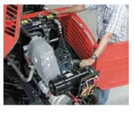
**Comfortable maintenance** PowerSwing<sup>™</sup> enables 360° access to both the engine and hydraulic system. For reduced downtimes and increased productivity.
