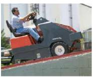
**Climbing Ability** Thanks to Power Climb<sup>™</sup>, PowerBoss's Armadillo is capable of climbing high curbs and inclines of up to 16% - in sweeping mode and with a fully loaded hopper.
