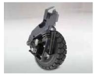
**Comfortable and robust:** PowerFlex<sup>™</sup>, the rear suspension – as used in the automotive sector – minimises vibrations for the driver and ensures a long service life of
