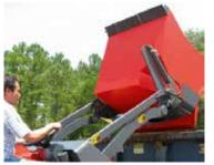
**Practical Feature** The robust sheet-steel debris hopper can be lifted to a dumping height of up to 64 in.
