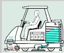
• The sweeping system picks up fine dust and coarse debris in the dry zone in front of the scrubbing unit.
