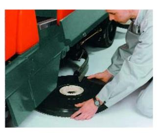
Excellent cleaning performance thanks to two directly driven disc brushes. Can be changed without additional tools. Up to 50% less water and cleaning chemicals used as a result of the Aqua-Stop-
