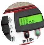
Machine Control Panel uses off-the-shelf toggle and marine duty switches and features universal icons which simplifies training.
