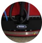
Squeegee Adjustments made simple with quick change squeegee latch allows tool-less maintenance and 4-sided squeegee blade.
