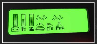
Operators quickly see bubbles on LCD display when Suds system is in operation. 6 total bubbles for "Single Dose" and 12 total bubbles for "Double Dose".
