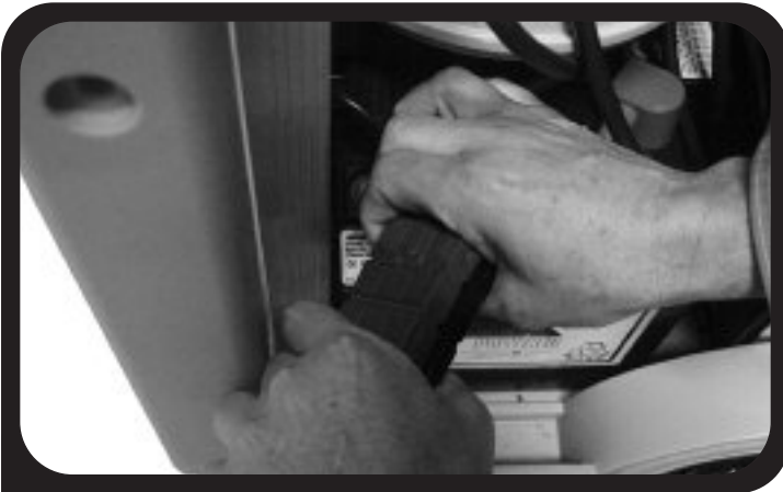
5a. Grab each end of the charging harness and work back and forth as you pull apart.
