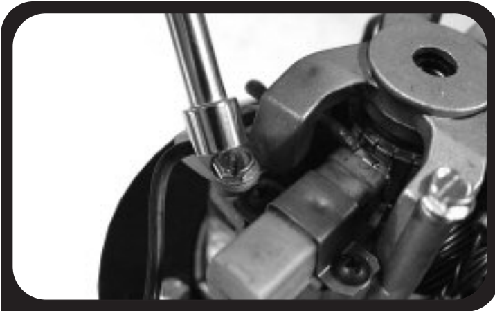
5a. Remove screw and wire retaining clamp on motor with 5/16" socket.
