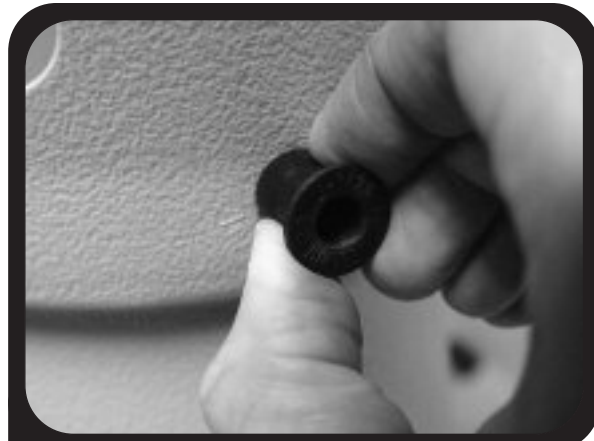
4. Press well nuts into holes in vacuum body. Rotating as pushing in may ease assembly.
