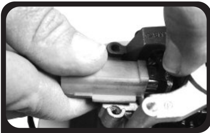
8. Remove motor brush. Remove 2nd motor brush in same way.
