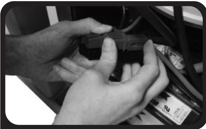
6a. Slide the charger's black/red connector apart from the other two.
