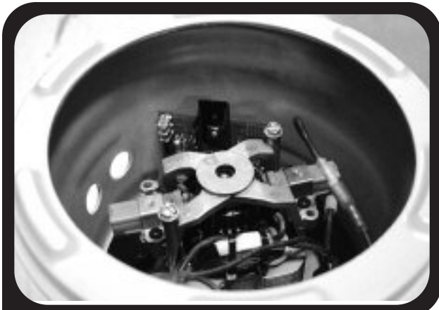
3. Align motor as shown in picture (BCM close to power cable hole).
