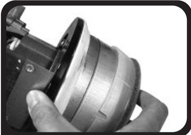
1. Press dome filter onto bottom of motor.
