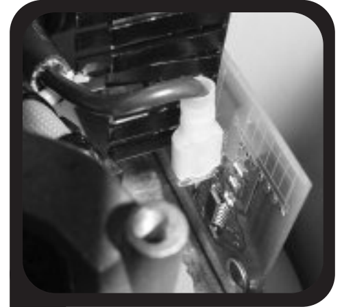
6. Locate black wire of power cable on BCM. Remove w/needle-nose pliers.
