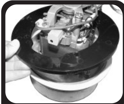
9. Remove ring over top of motor.
