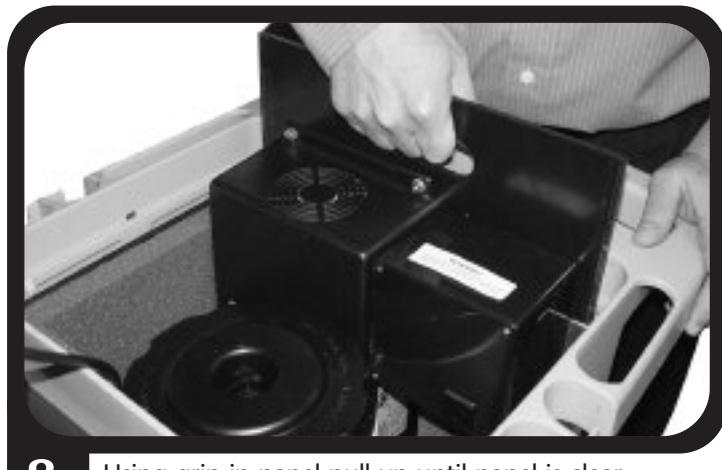
8. Using grip in panel pull up until panel is clear from cart.
