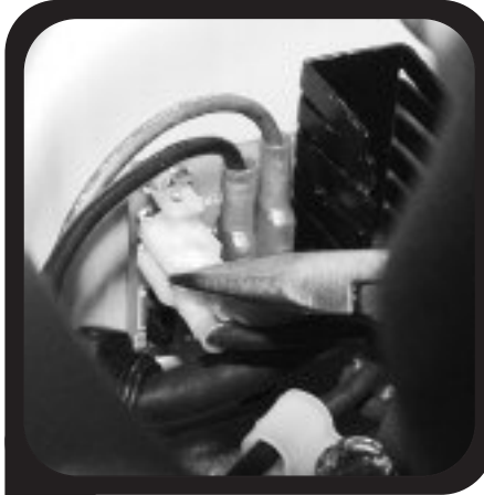
5. Locate white wire from power cable and remove from BCM.
