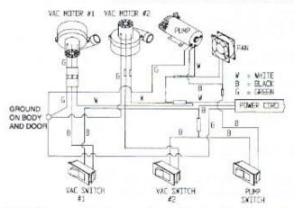
GREEN ground wire must be attached to the motor ground and to the body to properly ground the entire machine.
