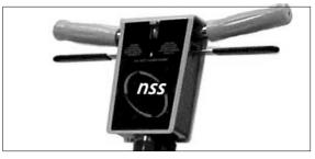
The Mustang features a mechanical lock-out on the handle which must be released before the switch lever can be activated. This important safety feature prevents unauthorized operation if the machine is left unattended.
