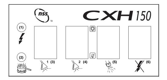
**CIRCUIT LOCATOR (1):** When this light is on, it indicates that cord #2 is on a
