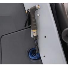
Apply solution to the floor in conjunction with vac wand, or used for machine cleaning. (optional)
