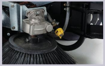
DustGuard<sup>™</sup> minimizes side broom fugitive dust generation and provides optimal sweeping performance. (optional)
