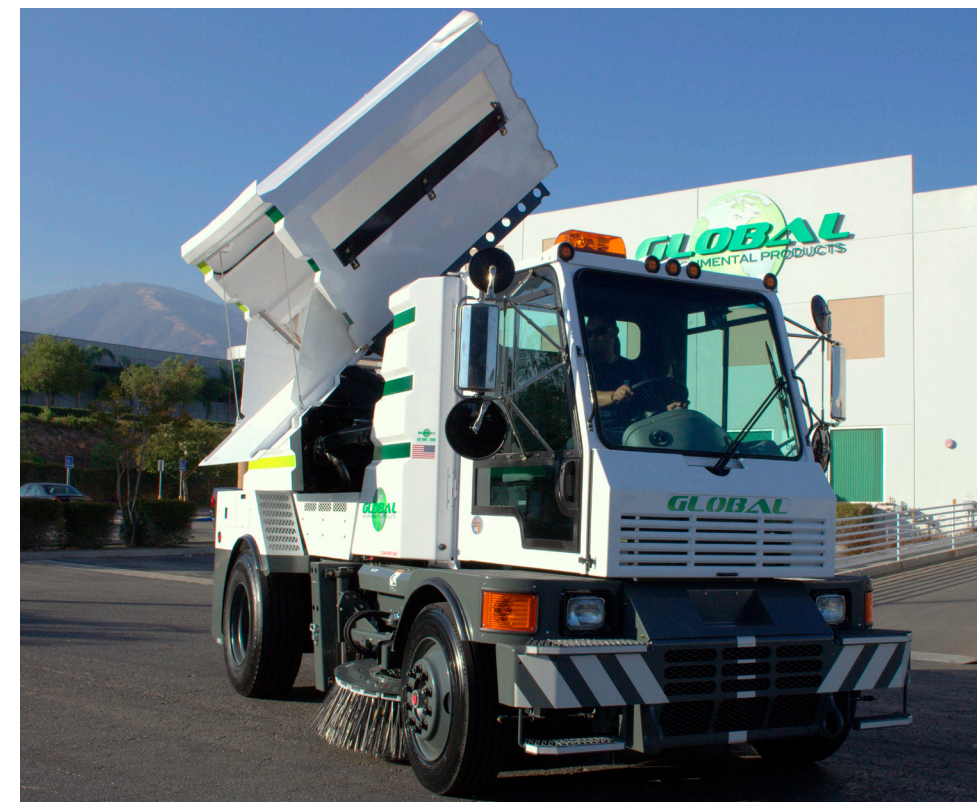
DUST SUPPRESSION SYSTEM consists of 280 Gallon Water tank & (2) Two Water Pumps rated at 3.5GPM @ 45Psi.
