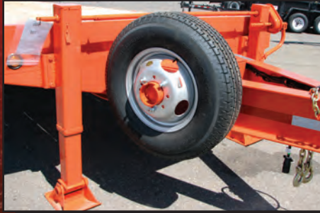
140K twin 2-speed jacks w/spare tire
