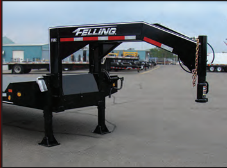
2 - 5/16" gooseneck coupler hitch
