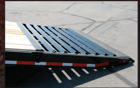
Angle iron on rear 1/4 of deck
