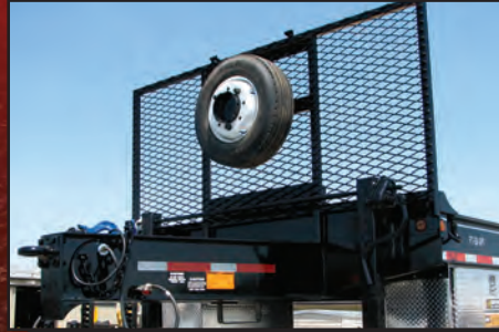
4' mesh headache rack w/spare tire
