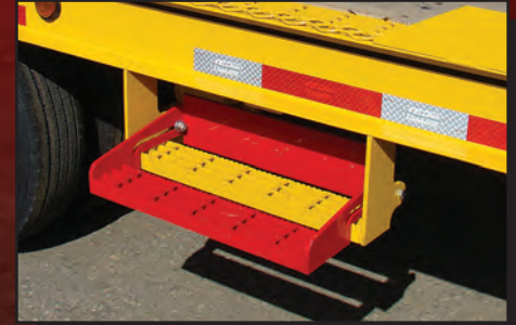
Bar grate step with pull-out extension
