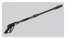
The spray gun has on/off spray control with insulated handle and two-piece insulated wand. The Multi-Reg spray nozzle adjusts from 0-60°, with high/low pressure adjustment for soap application. Variable spray pressure is adjustable at the pump.
