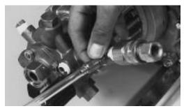
Chemicals are injected after the pump, so they can't cause problems to valves or seals. Ratios are set and locked in with controls by the operator. Chemical metering saves cost by reducing waste.
